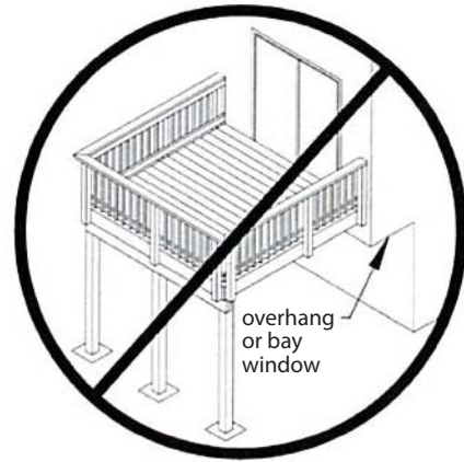
Figure 18. No Attachment to House Overhang
